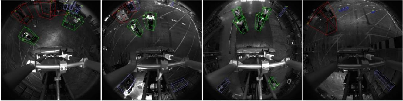
Fig. 9: Obstacle classification in different scenarios: Red – AGV, Green – Pedestrian, Blue – Other obstacle
