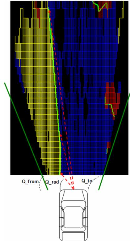
Figure 6: Border Scanning on the Occupancy Grid Points.
