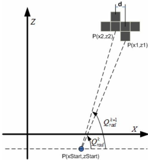
Figure 7: Radial angle estimation for the next step in the Variable Step Border Scanning approach.
