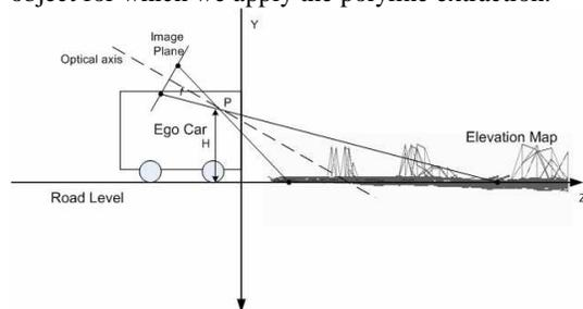
Figure3: The car coordinate system.
