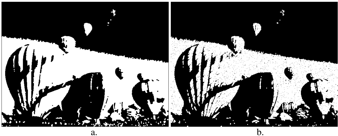
Fig. 7.8 Results of the opening (a) and closing (b) operations applied on the original image from Fig. 7.5a.
