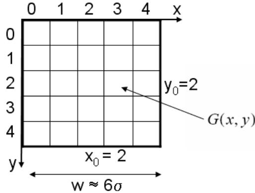
Fig. 10.4 Design example of a Gaussian kernel/filter having a 5x5 size.
